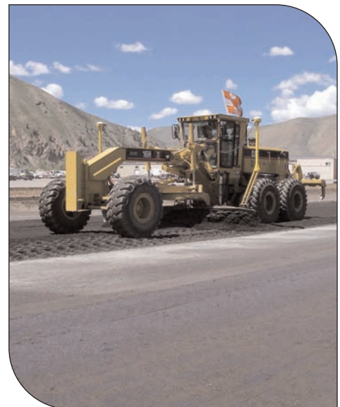
Grader with GPS technology.
